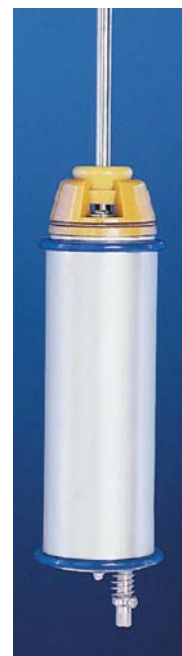
Figure 5.6. The Kemmerer discrete depth sampler capable of operation to depths of 180 m. Source: MDA Consulting Ltd. (2003)
